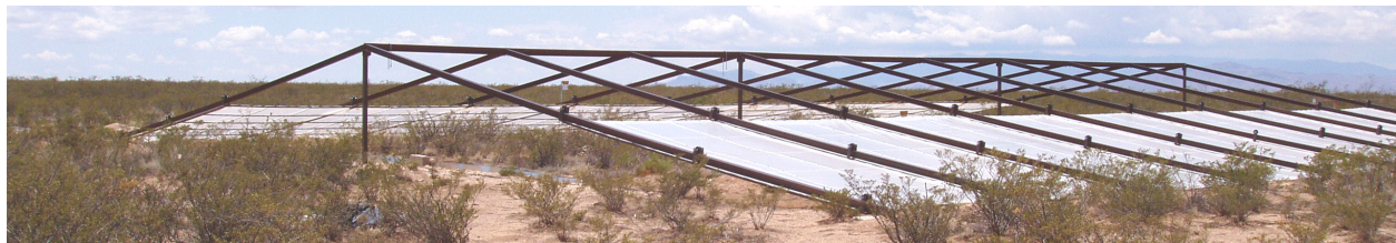
Fig 2. Rainout shelters in creosote-dominated shrubland. Similar shelters are located in black grama dominated grassland and in a grass-shrub transition zone. Water addition plots are located behind the rainout shelters.
